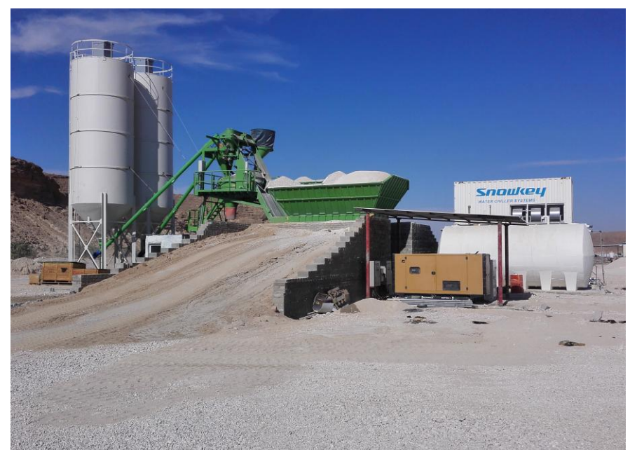
STETTER Semi Mobile Plant : Erected in 2016 Capacity 56m 3 /hr.
